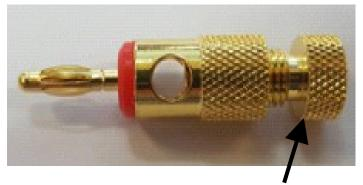
Turn retaining screw anti-clockwise to reveal hole
