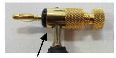
Insert 4mm banana plug into hole, ensuring a good contact between plug and adaptor
